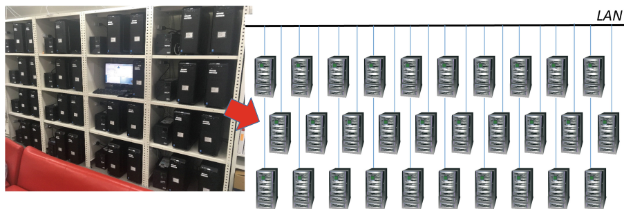
30 × CPU Core i7 5820K 6core/12thread 3.3GHz 64GB RAM
