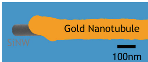
Fig. 6.16 Gold nanotubes made from silica nanowires. The figure shows the silica nanowire (SiNW) core and the gold nanotube coating. (Reprinted from Guo et al. [62]. Copyright (2006), with permission from Elsevier.)
