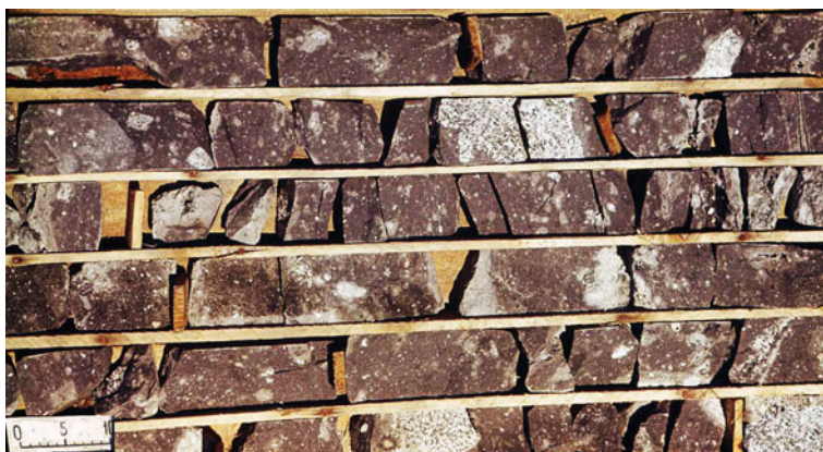
Fig. 4.5 LT tagamite with numerous inclusions of gneisses (light-colored), which are shocked to a variable degree and annealed. Mayachika Upland, borehole 1726, depth 42–48 m. Core diameter is 57 mm. The scale on the figure is in cm
