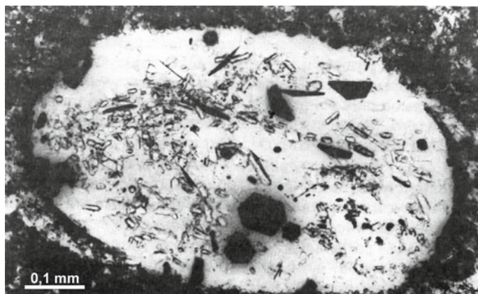
Fig. 4.14 The spheroid of pyrometamorphic glass in HT tagamite. Microlites of plagioclase, hypersthene, ilmenite are visible in the partially crystallized glass, which in places shows trachytoid texture. Microphotograph, parallel nicols
