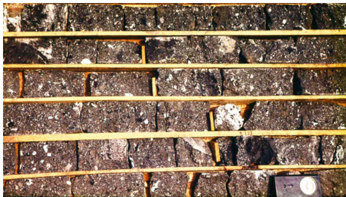
Fig. 4.18 The core of lithovitroclastic suevite. The xenomorphic lapilli-sized gneiss fragments (light), as well as fragments of argillites and siltstones (dark grey) are cemented by groundmass of fine-grained glass particles. Mayachika Upland, borehole 1726, depth 123.7–137.6 m. Core diameter 46 mm
