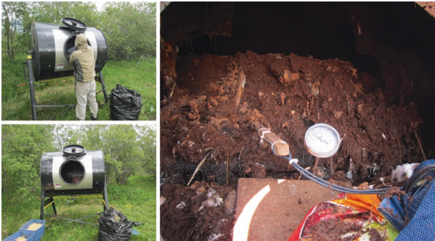
Fig. 20.3 Continuous flow batch composter (Actium, Seaforth, ON, Canada) with a manual crank and capacity of 1.6 m 3 or 682 kg of material. High density fiberglass insulated with an ultraviolet resistant jacket
