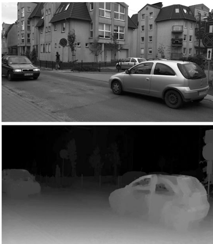
Fig. 2.2 A view and the corresponding depth map from the test multiview sequence Poznan_Street [34]
