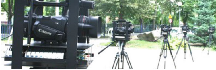
Fig. 2.16 Tripods with wireless camera modules designed and produced at Poznań University of Technology © IEEE 2016
