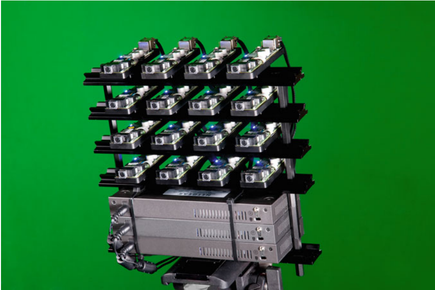
Fig. 2.8 16-camera full parallax camera array of Fraunhofer IIS. Copyright: Kurt Fuchs| Fraunhofer Institute for Integrated Circuits IIS
