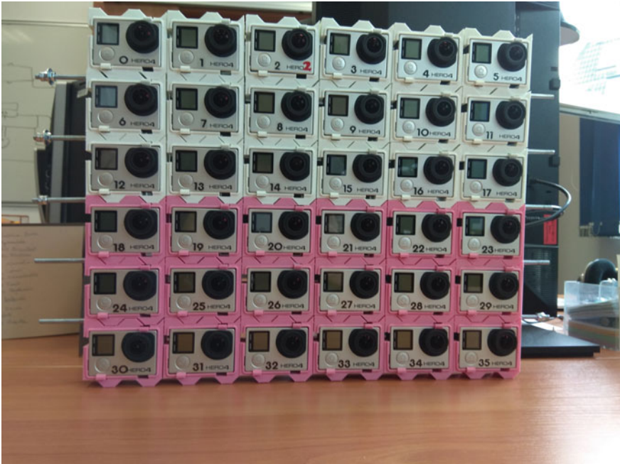
Fig. 2.9 36-camera matrix at Poznan University of Technology, Multimedia laboratory
