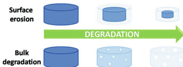
Fig. 8 Degradation mechanisms; surface erosion versus bulk degradation
