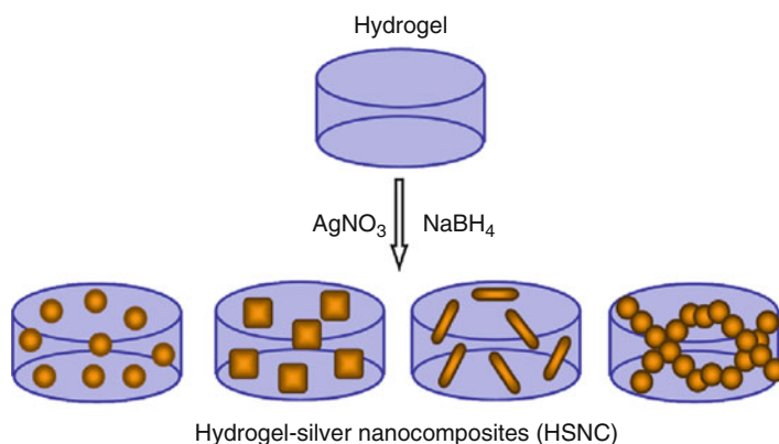
Fig. 15 Hydrogel networks used as templates to synthesize of silver NPs [239]
