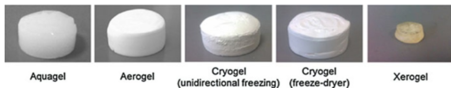
Fig. 10 Examples of an aquagel and samples after drying with different techniques (aerogel, cryogels, and xerogel) obtained from 7 wt% cellulose solution. (Reprinted with permission from [63]. Copyright © 2016, Springer International Publishing AG.)
