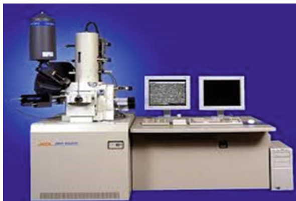
Fig. 8 Photographic image of the scanning electron microscopy instrument
