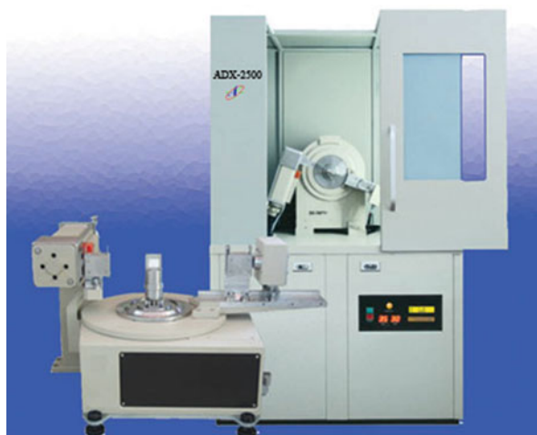
Fig. 6 Photographic image of the X-ray diffraction analysis instrument
