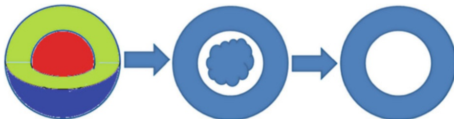
Scheme 3 Schematic illustration of the transition of chitosan hydrogel in the deposition process. (Reproduced from Hao et al. [45], copyright © 2016, with permission from Elsevier Inc.)
