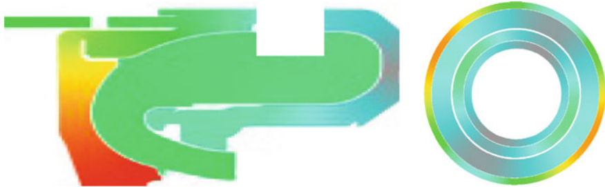
Fig. 7 Pressure fluctuation modulus field. Left—first longitudinal mode (490 Hz); right—first azimuthal (standing) mode (680 Hz)
