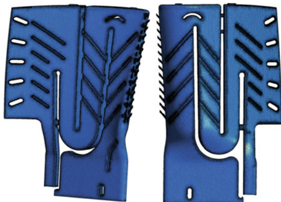
Fig. 3 Internal cooling passages mesh
