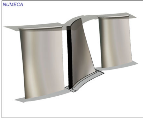
Fig. 3 Computational domain for the 1.5-stage high-pressure compressor
