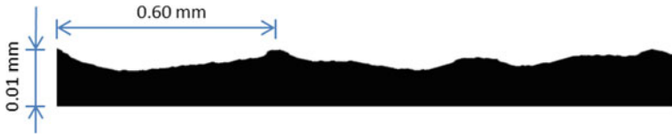
Fig. 5 Exaggerated actual surface measurement with high resolution for the second- and third-order shape deviations. Only by exaggerating the deviation in the normal direction of the surface, these deviations from machining turn visible
