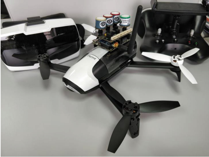
Fig. 2. Parrot Bebop 2 FPV drone with Wasmote sensors
