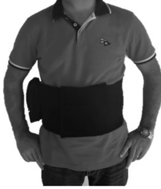
Fig. 2. Gait detection system developed on a waistband: the bag on the left houses the processing unit and the data storage system, whereas the gait acquisition system, the IMU, has been embedded so as to be placed in T2-L1 inter-vertebral space.
