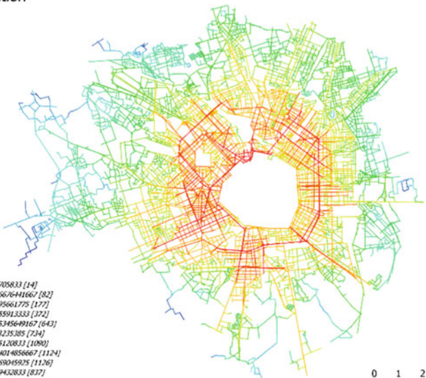
Fig. 9 Integration map of vehicular accessibility and potential location of park and rides (first image); integration map of vehicular accessibility based on prohibited traffic zone (second image)
