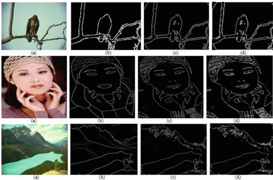
Fig. 5 Visual results of QGA and comparison. (a) Original image. (b) Ground truth. (c) Canny edge. (d) QGA edge
