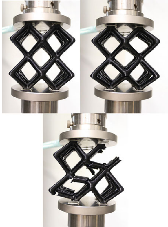
Fig. 3 Compression testing of the lattice bricks
