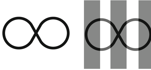
Fig. 3. Line following task. On the left the road that the agent must follow. On the right the same road path with different friction areas.
