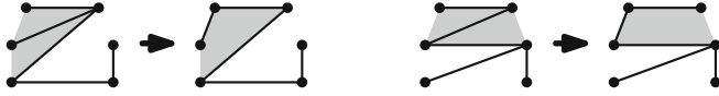
Fig. 4. Small cells of degree 2 are merged by one slide only involving the parent edge.
