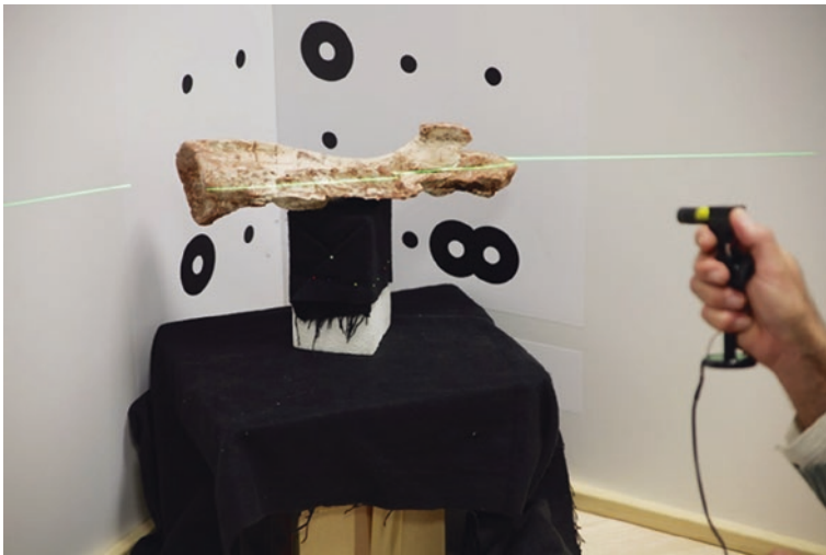
Fig. 2.3 Scanning process, the technician scans the object by moving the laser-scanner. Image: State Museum of Natural History in Braunschweig
