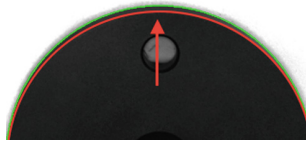
Fig. 6. Actual outline. Red edge is the actual flange front outline, and green edge is a side-view contour. (Color figure online)
