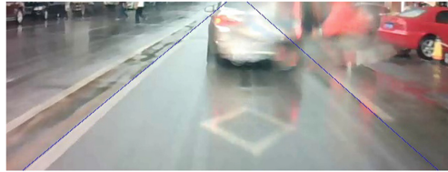
Fig. 6. Lane detection results. The blue line is the detected lane. (Color figure online)
