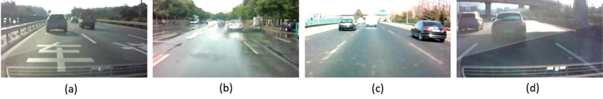
Fig. 1. Images of advanced driver assistance system. In (a), road is full of noises. In (b), in the rainy day, the lane is very blurry. In (c), the lane is worn. In (d), there are variant lighting conditions.
