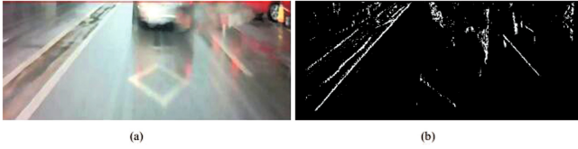
Fig. 3. Result of Algorithm 1. (a) is the source image under the rain. (b) is the result of Algorithm 1. We can find lane structure from (b).
