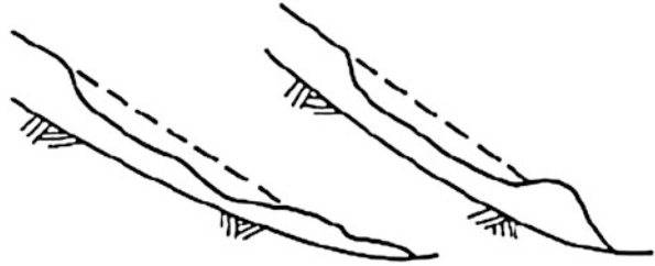
Fig. 2.20 Shallow flow slide failure
