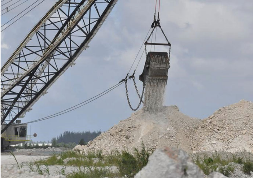
Fig. 2.11 Dragline dumping the overburden material in an opencast mine [17]
