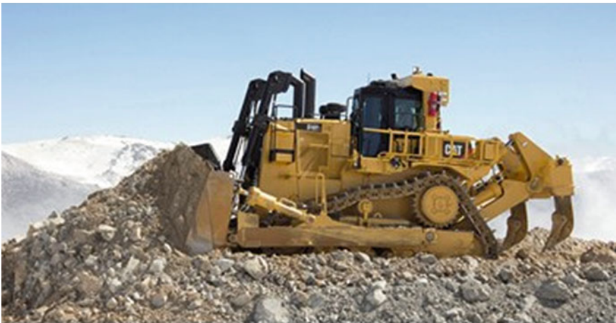
Fig. 2.9 Dozer push dumping the overburden material in an opencast mine [15]
