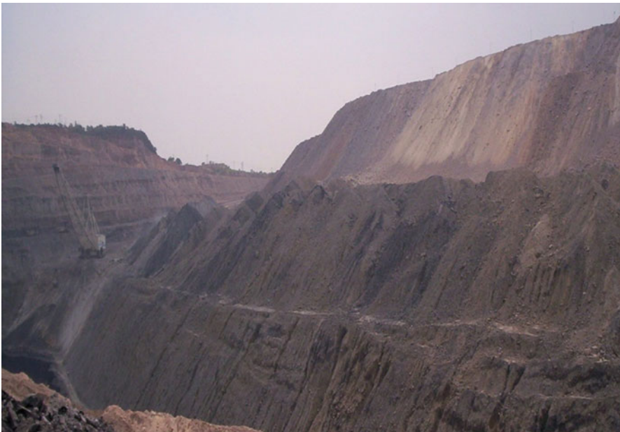
Fig. 2.1 A typical internal dump in one of the coal mines in Northern coalfields limited
