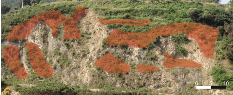
Fig. 5.11 Map of the unstable sectors of the slope showing the potential evolution of the instability [12]
