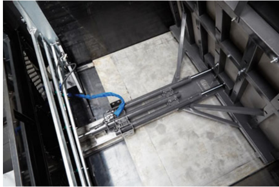
Fig. 3.13 The hydraulic cylinder and installation that moves the push-off wall [Fliegl Agrartechnik GmbH]
