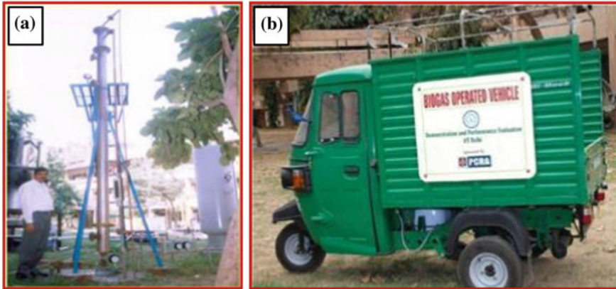
Fig. 18.1 Demonstration model installed at IIT-Delhi; a biogas scrubbing system and b biogas operated three wheeler
