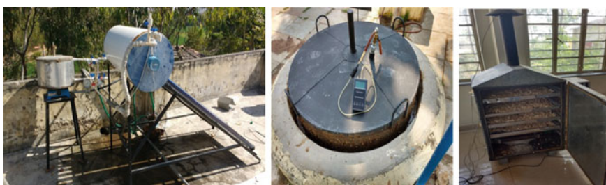
Fig. 18.3 Hybrid solar/biogas dryers for button mushrooms
