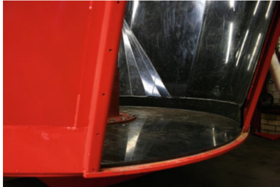
Fig. 3.16 Special polyethylene coating to protect the carbon steel frame [Trioliet B.V.]
