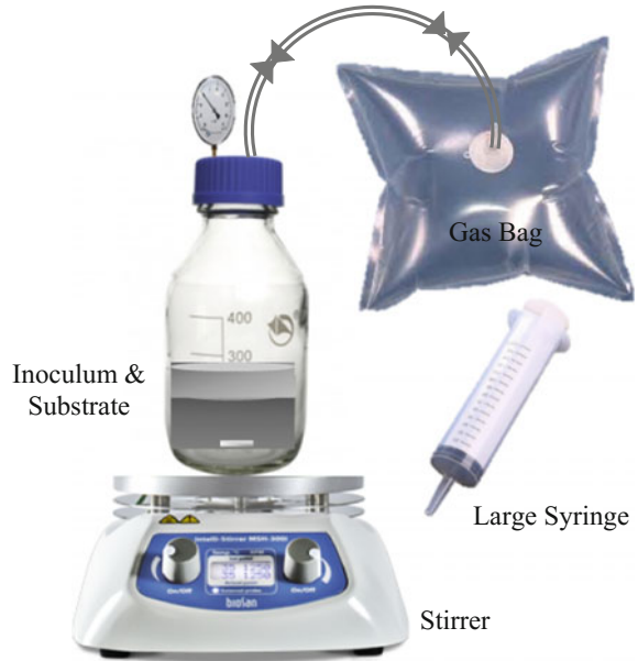
Fig. 9.5 The illustration of the large syringe at intervals method. The apparatus should be placed in a climate chamber at a desired temperature
