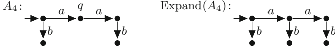
Fig. 3. On the left: The lts A_4 with \text{SSP}_{\text{unsol}}(A_4) = \emptyset and \text{ESSP}_{\text{unsol}}(A_4) = \{(q, b)\} . Because there are no unsolvable state separation problems, A_4 and \text{Merge}(A_4) are isomorphic. On the right: The lts \text{Expand}(A_4) where a new edge with [q][b] was added.
