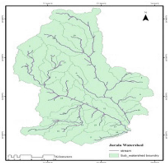
Fig. 2 Schematic diagram of Jurala watershed (Sub watershed and streams are delineated from SRTM DEM)
