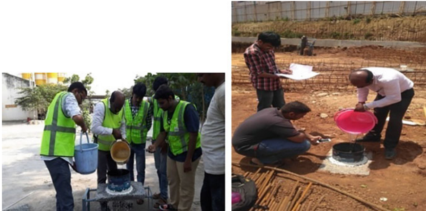
Fig. 8 Laboratory test and field test with and without soil surface through pervious concrete
