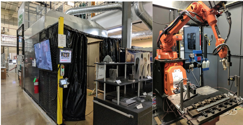
Fig. 3. mBAAM protective wall (left) and the robotic manipulator with printing head and wire feeder (right)
