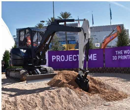
Fig. 7. 3D printed excavator during CONEXPO 2017 demo tests
