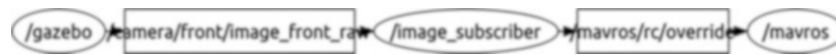
Fig. 73.11 Diagram generated by the program rqt graph showing the relevant nodes and topics in the application
