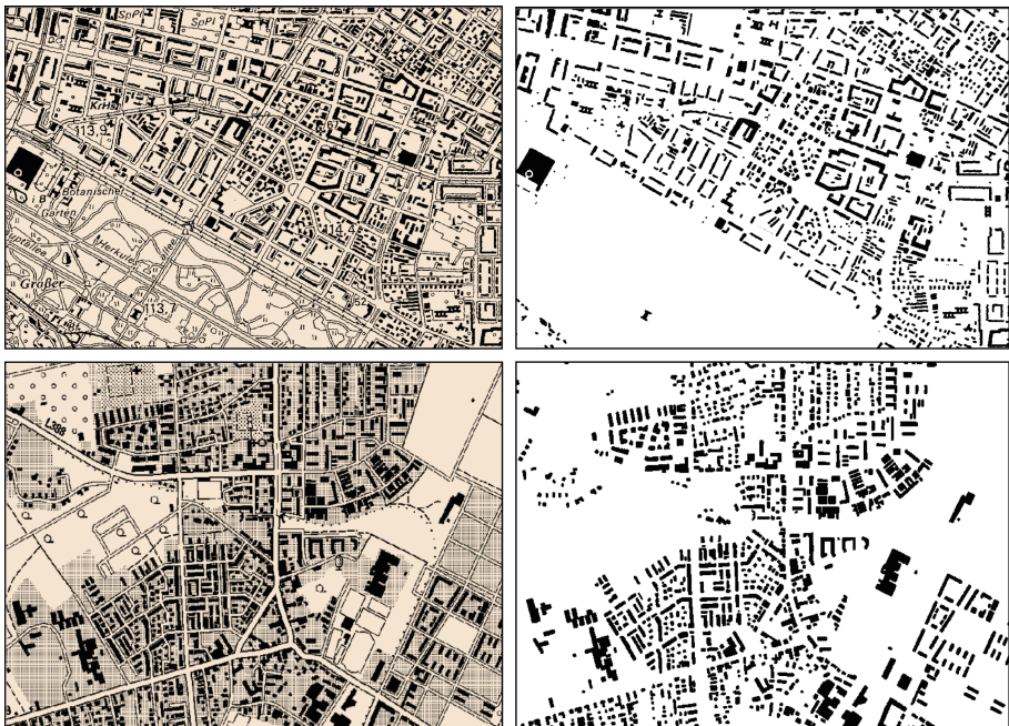
Fig. 3. 2D building extraction from topographic maps (map data sources: TK25 © GeoSN 2006 for the map on the upper left, TK25 © GeoBasis NRW 2005 for the map on the lower left).
