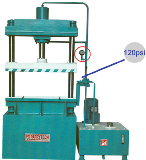
Fig. 4.3 Registration errors cause the real and virtual objects to be misaligned. The pressure dial (real) does not align with the virtual indicator
