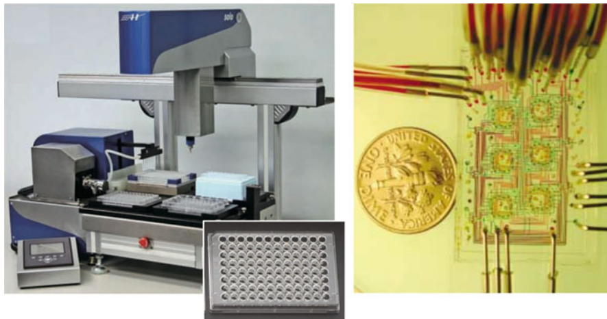
Fig. 11.2 Automation and cost reduction in life-science experiments via (left) liquid-handling robotics and (right) microfluidics. (Images adapted from Kong et al. (2012) and Balagaddé et al. (2005))
