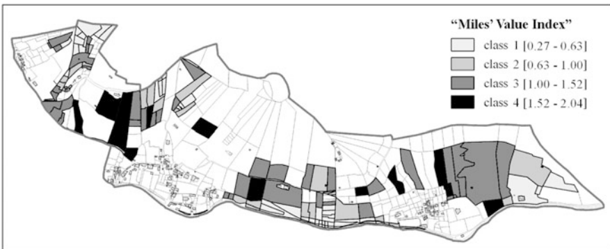
Fig. 7 Ranking and classification of abandoned cadastral parcels in terms of rehabilitation suitability according to the Miles' Value Index method. Source: Bonelli (2017), modified
