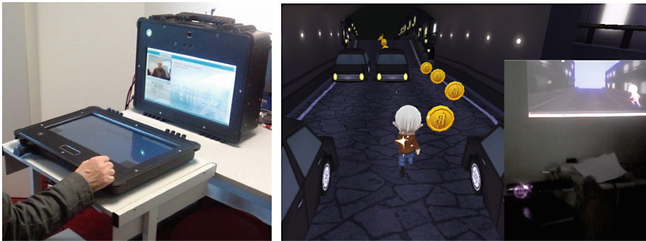
Fig. 6. Virtual Table for limb training (left) and “Endless Runner” game executed on it (right)
