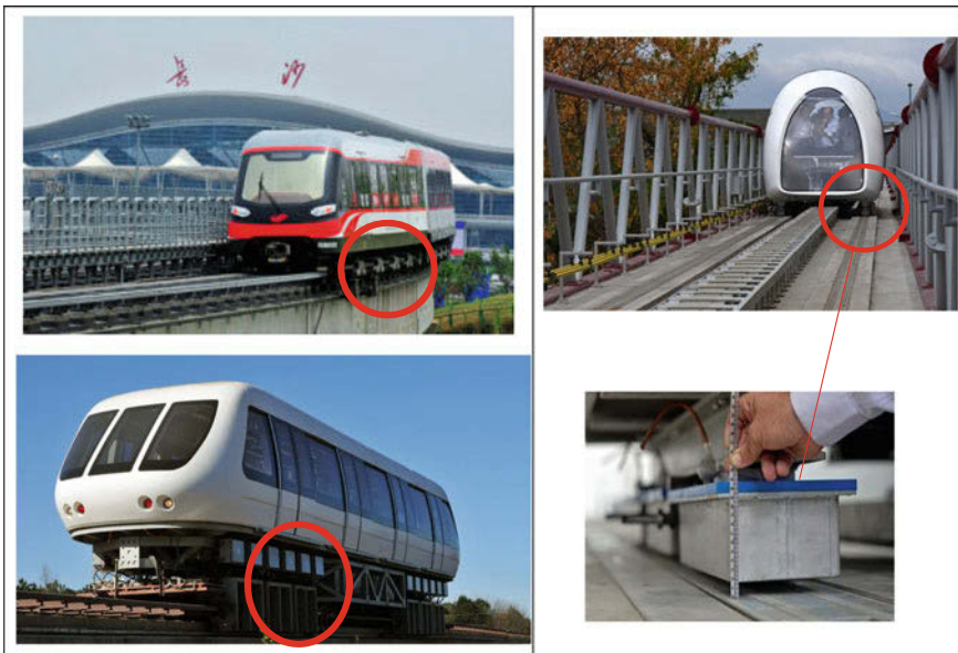
Fig. 5 Comparison of the equipment necessary to achieve EML (left side) with the cryostats necessary for the MagLev-Cobra (SML) project (right side): simpler and more robust
