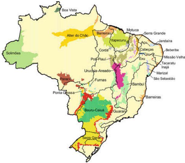
Fig. 2 Schematic representation of the main Brazilian aquifers and their extensive recharge areas (Agência Nacional de Águas 2005)
