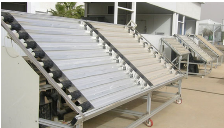
Fig. 4 View of several solar CPC pilot plants located at Plataforma Solar de Almeria, The Solar Research Centre in Spain
