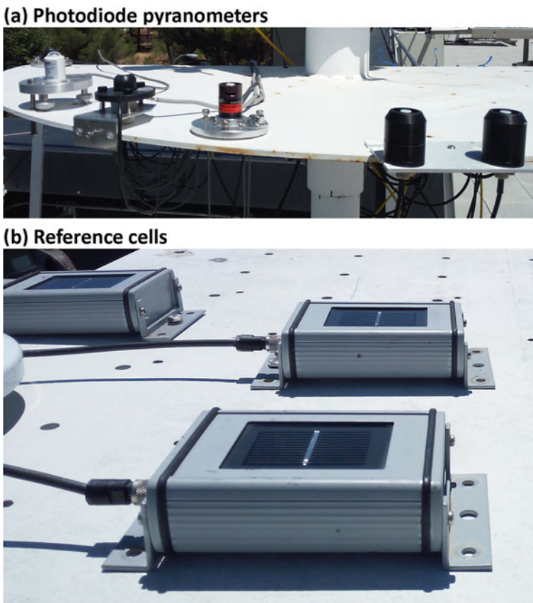
Fig. 9 Silicon-based sensors for measuring solar radiation
