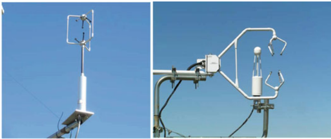
Fig. 5 Two different types of sonic anemometers to measure the three components of wind
