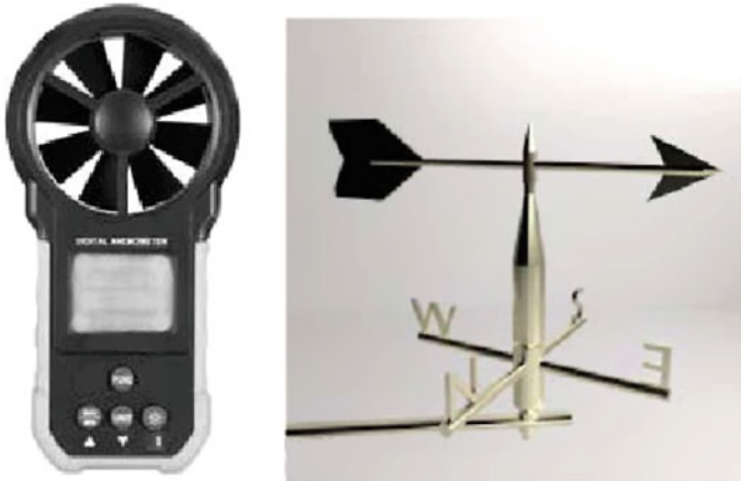
Fig. 1 Left. Handheld anemometer which should face directly to the wind. Right. Simple vane indicating where the wind comes from
