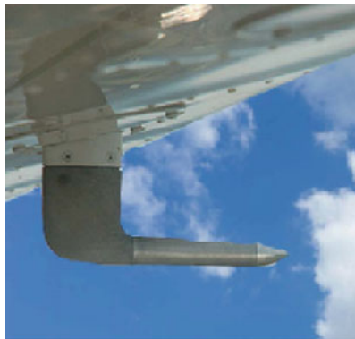
Fig. 3 Pitot tube anemometer mounted in an aircraft
