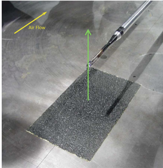
Fig. 2 Photograph of a rough patch panel and sound intensity probe above the patch. Scans were made in the flyover direction along the flow
