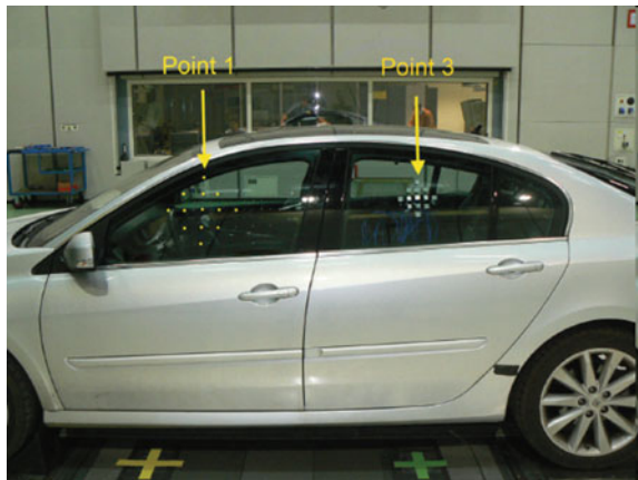
Fig. 10 Photography of the Renault Megane car used for the identification of acoustic wall pressures when the car is placed in a reverberant room
