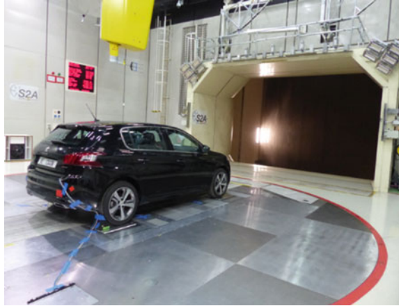
Fig. 13 Photography of the PSA 308 car placed in the S2A wind tunnel
