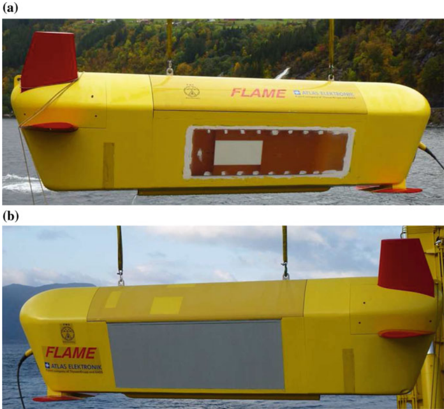
Fig. 2 Flow Noise Analysis and Measurement Equipment (FLAME) towed body with two different flat plate configurations: sandwich plate (brown rectangle) with measurement area (inner white rectangle) on starboard side (a) and flat plate area (gray rectangle) with embedded hydrophone array on port side (b) of the towed body
