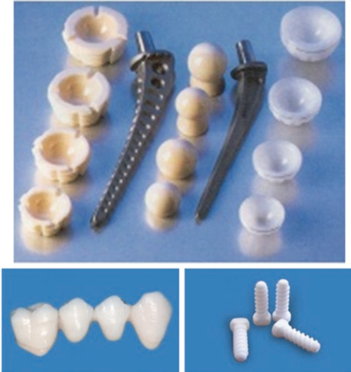
Fig. 3.2 Bioceramics of alumina and zirconia used for orthopedics and dentistry applications [30, 31]
