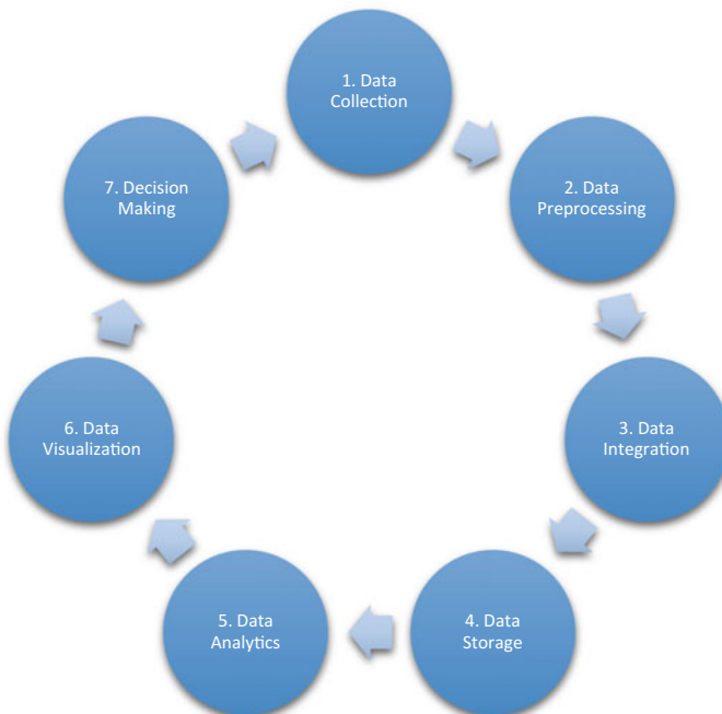
Fig. 8.1 Energy data life cycle for smart grids
