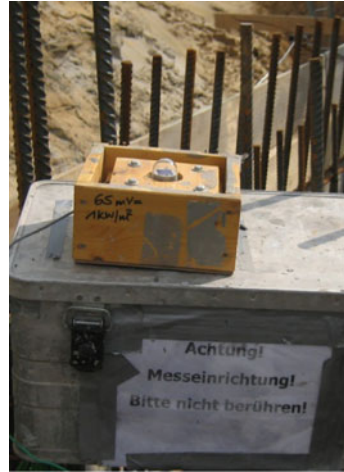
(b) self-built device on basis of a solar cell (photo: D. Schlicke)
