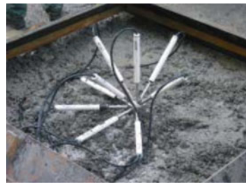
(d) Carlson strain gauges being grouped by a spider (Mata et al. 2015)
