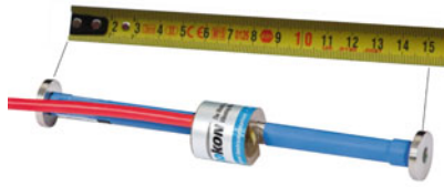
(a) "pure" vibrating wire sensor according to (Geokon, 2017)
