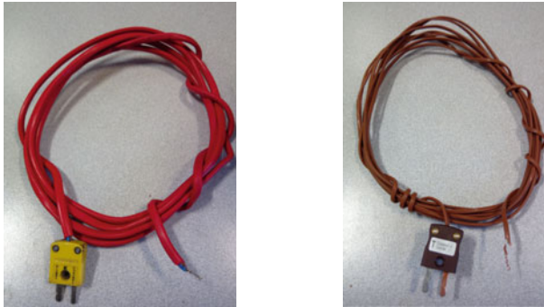
(a) Type K thermocouple wire (b) Type T thermocouple wire
