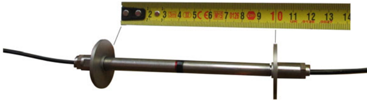
Fig. 9.21 Fibre optical concrete embedment strain gauge on basis of fibre Bragg technique (Photograph D. Schlicke)
