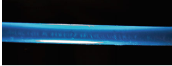
Fig. 3 Experimental image showing the onset of a helical instability along a biofilm thread in a 2 mm diameter tube
