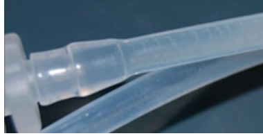
Fig. 2 Experimental image showing a biofilm helix wrapped around the tube wall past the junction. No biofilm is formed in the unperturbed branch. Bacteria were injected upstream the junction
