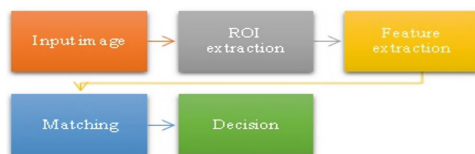
Fig. 1. The process of the dorsal hand veins recognition.
