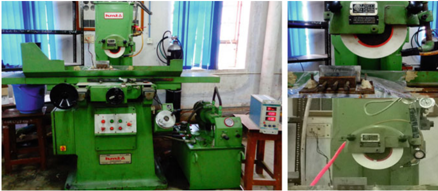
Fig. 1 Setup for soap water jet application, and liquid CO 2 assisted soap water jet application
