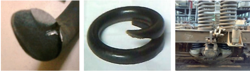
Fig. 1 Photographs of failed primary inner spring and arrangement of middle axle suspension spring near middle wheel
