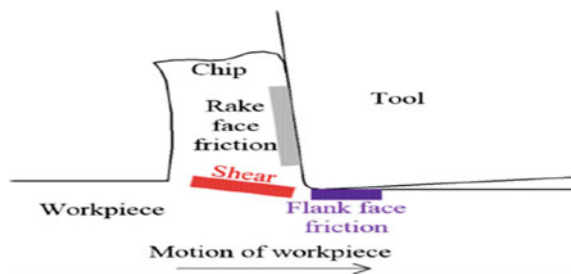
Fig. 2 Heat sources in machining referred from Chen Lei et al. [10]
