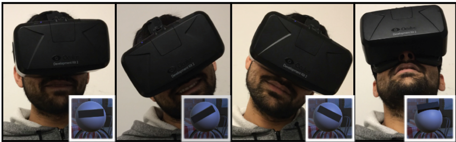
Fig. 6. Audience avatars in the virtual space which move based upon the head motion of the audience member watching in the physical space
