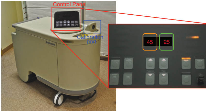
Fig. 9.2 Excimer laser generator (Spectranetics® Colorado Springs, CO, USA). The Spectranetics CVX-300 system system which is a portable unit 89 cm high, 124 cm long and 61 cm wide weighing approximately 295 kg. The system can emit laser energy from 30–80 mJ/mm 2 (indicated within the orange panel) with repetition rate from 25 to 80 Hz (indicated in green) and a pulse
