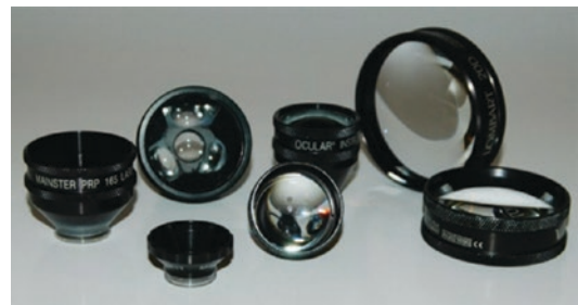
Fig. 2.6 Commonly employed ophthalmic lenses. A multitude of lenses can be used for argon laser treatment application depending on the desired magnification and field of view. Such lenses can be broadly categorized as either corneal contact lenses (five lenses located on the left: ocular Mainster 165, ocular three mirror, ocular Yannuzzi fundus, ocular Reichel-Mainster and ocular Mainster wide field) or indirect lenses (two lenses located on the right: 20-diopter and 28-diopter)
