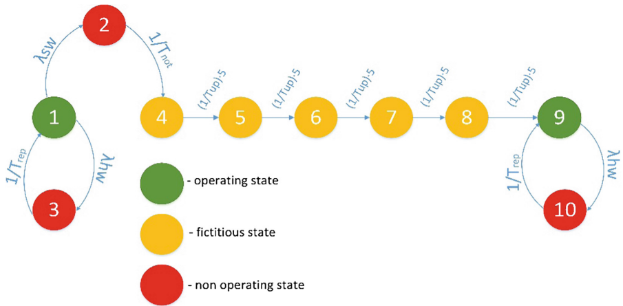
Fig. 5. Fragment of Markovian chain with describe operations critical NPP I&C system and 5-phase Erlang distribution of software update
