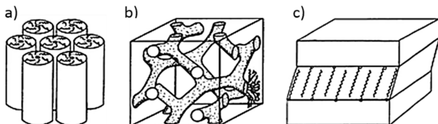
Fig. 3.2 Different types of mesoporous materials. (a) Hexagonal arrangement of pores: type Mobil Composition of Matter-41 (MCM-41); (b) Cubic arrangement of pores: type MCM-48; (c) Lamellar arrangement of pores: type MCM-50. Reprinted with permission of the Royal Society of Chemistry from (Corma et al. 2008)
