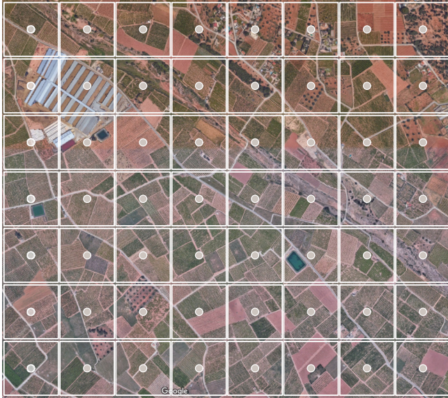
Fig. 1. Example of a discretized area, calculating the tiles and their center to restrict movements.
