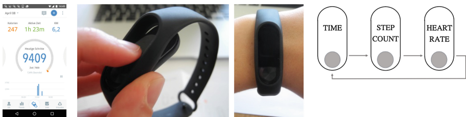
Fig. 1. A screenshot from the pedometer smartphone app (Pacer), the fitness tracker (Mi Band 2), and the toggling cycle for display content on the fitness tracker.
