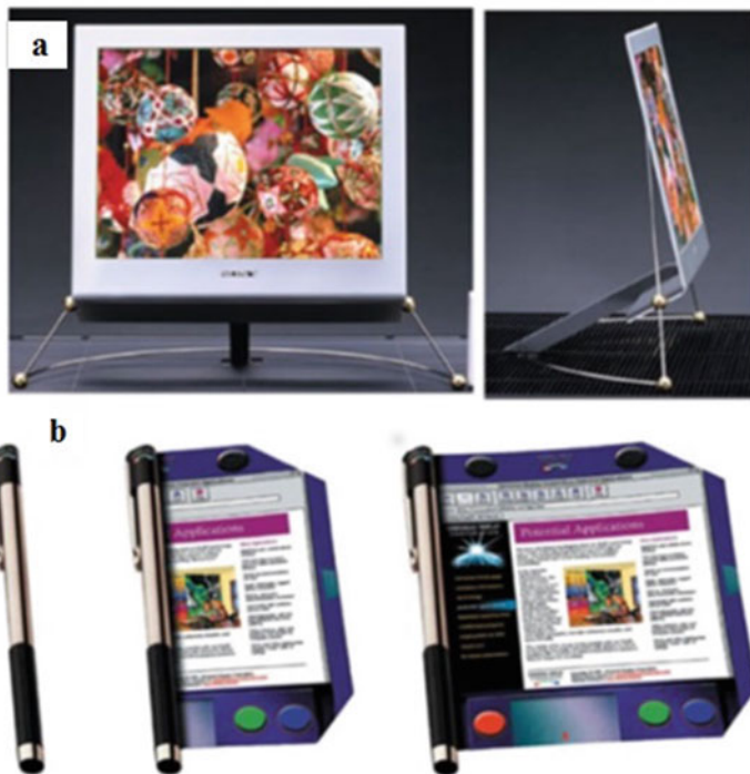
Fig. 1.19 (a) 2-mm-thick OLED monitor and (b) Concept for a future OLED screen, which could be rolled up like a scroll inside of a pen-sized device when not in use (Reproduced from Forrest 2004 Copyright (2004) Nature Publishing Group)
