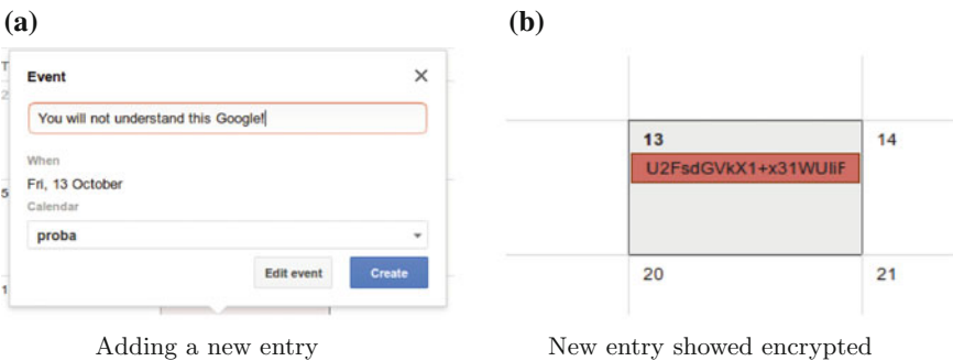
Fig. 5 Adding a new entry that is automatically encrypted on client side, and shown in the calendar without decryption
