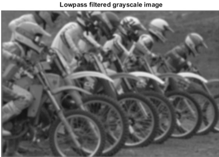
Fig. 4.18 Image in Fig. 4.12 filtered through the lowpass FIR filter of Fig. 4.11. The effect of lowpass filtering is to smudge the image as is evident from the figure
