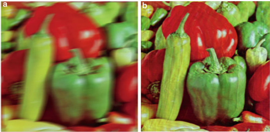
Fig. 1.7 An example of image deblurring. (a) Original blurred image. (b) Restored image
