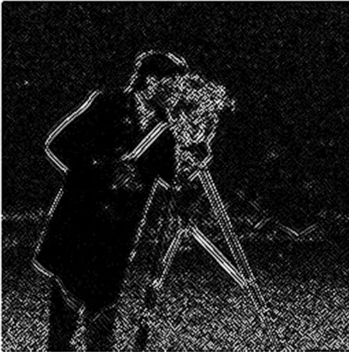
Fig. 7.52 Highpass filtered Cameraman image using the 2D highpass FIR filter of Example 7.14
