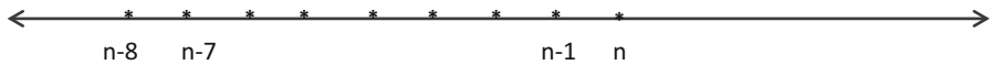
Fig. 9.13 Block of eight samples used to calculate the SDFT at time indices n and n-1
