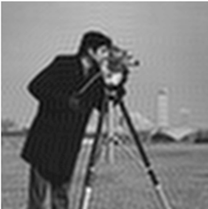
Fig. 9.28 Reconstructed image of cameraman by using only the first 64 \times 64 2D DCT coefficients. The resulting SNR is 11 dB
