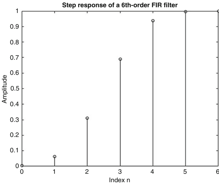
Fig. 3.12 Step response of the FIR filter of Example 3.17 as a single section
