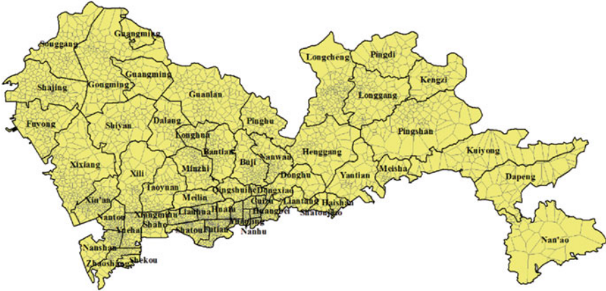
Fig. 9.1 Base station region (BSR) by Voronoi. Fine line is the boundary of the BSR and coarse line is the boundary of the district region in Shenzhen
